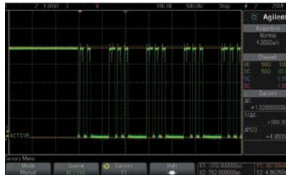
b) The output measured with an active probe with 1-MΩ input impedance makes the amplitude measurement correctly.
