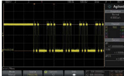
a) The amplitude of the signal measured with the 100:1 resistor divider probe is decreased to 1.65 V due to the resistive loading of the low-impedance probe.
