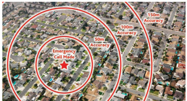
A typical E911 call from a mobile phone can pinpoint the caller’s location to within 50 m, translating to about 27 houses in this type of neighborhood.
